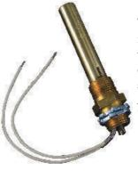
The adjustable thermostat is factory set at 95°F (35°C). It will normally hold ±2°F (1°C) of the desired temperature setting. It is rated 24V-240V AC or DC, 50/60Hz and is UL Recognized, CSA Certified.
