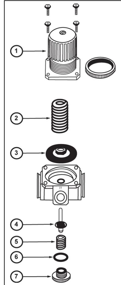
If leaks persist, remove bonnet, inspect diaphragm and diaphragm seat for wear or foreign materials.
